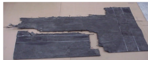
Weft Cord Located Above the Warp Steel Cord Flexible Cord Ensures Conveyor Belt Troughability Weft Cord (Figure 2)
